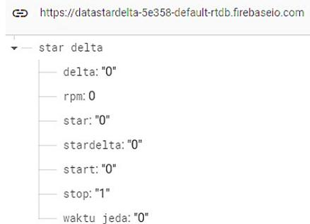
Gambar 13 Database Variabel Kontrol Motor
