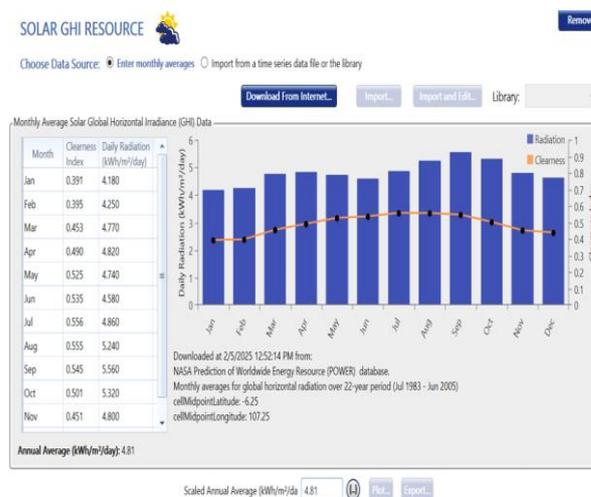
Gambar. 3 Diagram data *Solar Global Horizontal Irradiance* (GHI) bulanan
