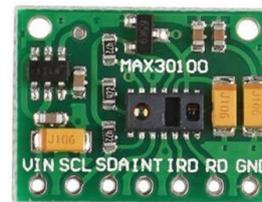
Gambar 1. Sensor MAX30100 [maximintegrated.com]
