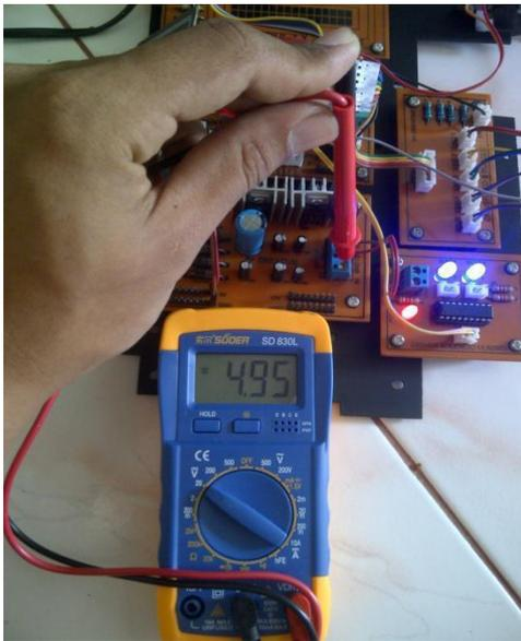
Gambar 15 Tegangan Output Power Supply 5V
